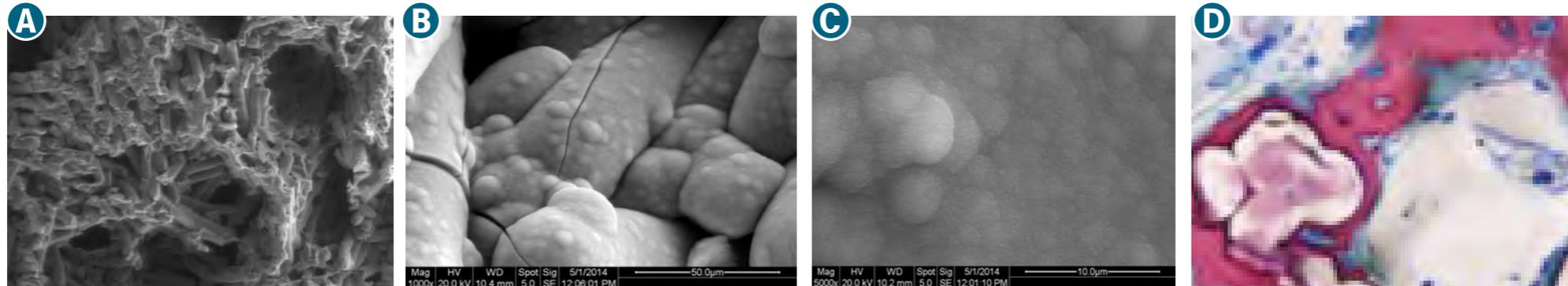
**A** Vitrium features an interconnected porosity with both micro and interconnected macropores providing a large surface area of material to interact with the body. The ensuing hydrolytic process results in the release of Na, P, Ca and other ions and the elevation of pH to create a beneficial chemical environment for the formation of new bone.
